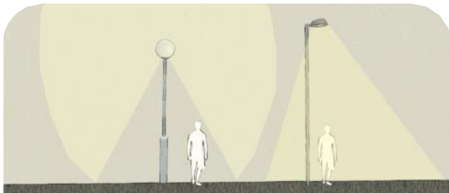
Fig. E5.1 Light on the left is not shielded; light on the right is shielded to direct light downwards only
